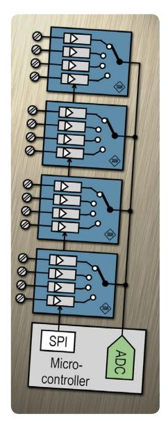
The Specific Component includes functions for configuration for different sensor types. It also includes analog signal processing functions as well as hardware to multiplex the measurement readings to the analog bus.
